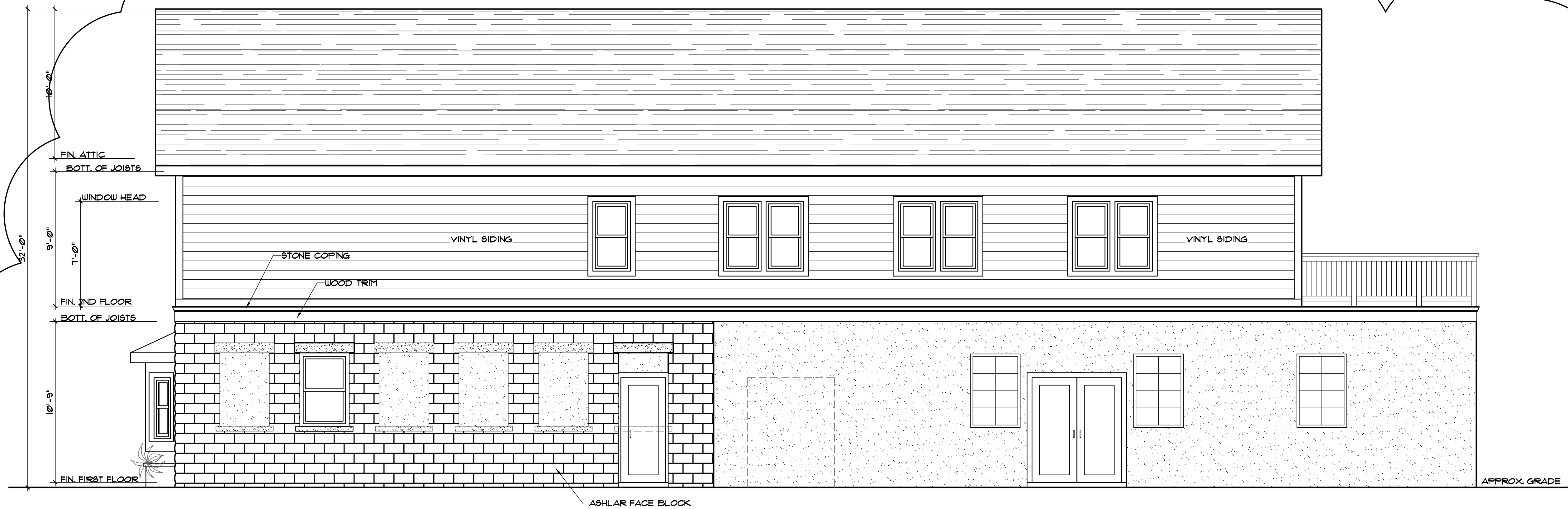
1 AR-4 PROPOSED RIGHT SIDE ELEVATION SCALE: 1/4" = 1'-0"
