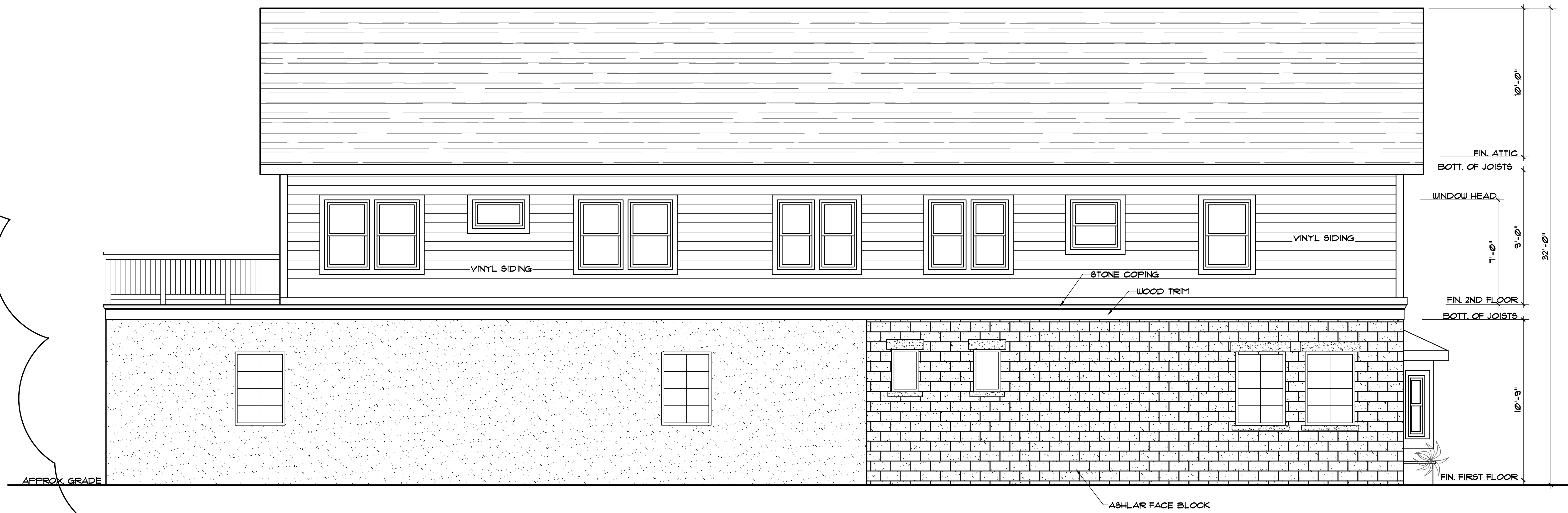
2 AR-4 PROPOSED LEFT SIDE ELEVATION SCALE: 1/4" = 1'-0"
