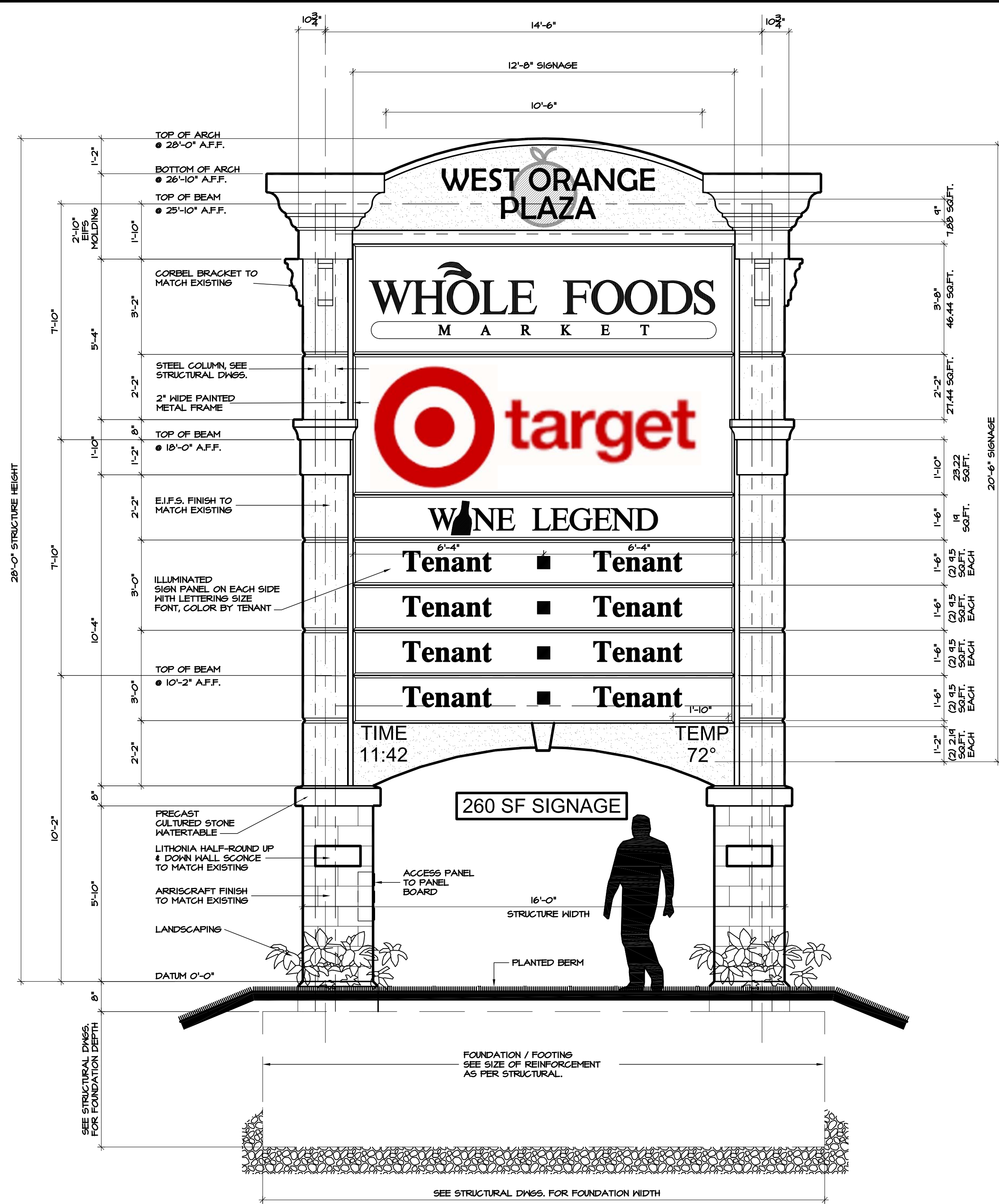
1 PYLON SIGN at SOUTHERN PROSPECT AVENUE ENTRY SCALE: 1/4" = 1'-0"
