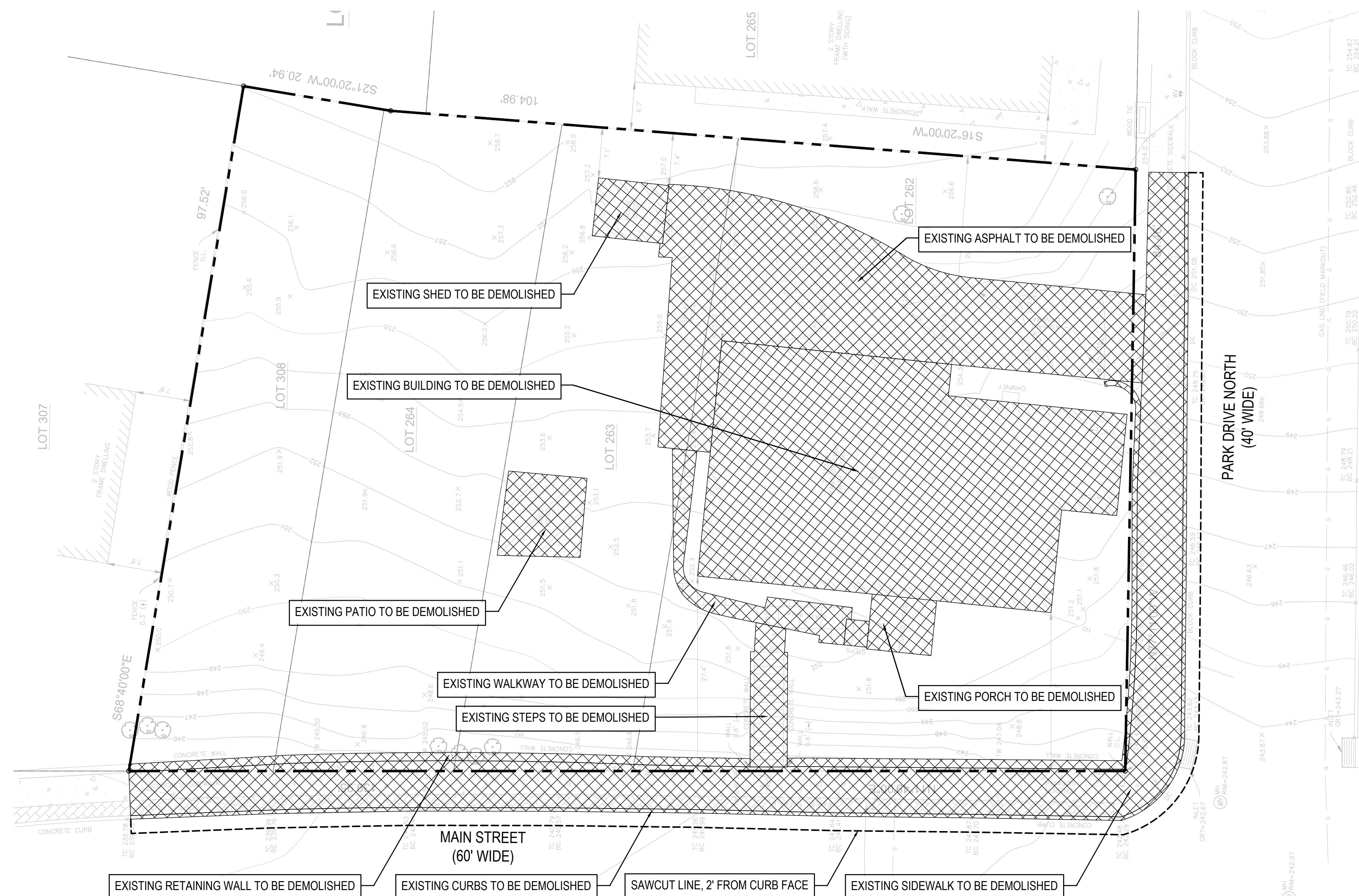
1 EXISTING CONDITIONS & DEMOLITION PLAN 1" = 10'
