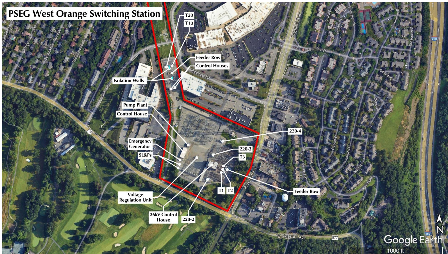
Figure 1 — Aerial photo showing existing conditions at PSE&G West Orange Switching Station, West Orange, NJ. Also labeled are existing major equipment. The site property line is outlined in red. Existing isolation walls are shown in light blue.
