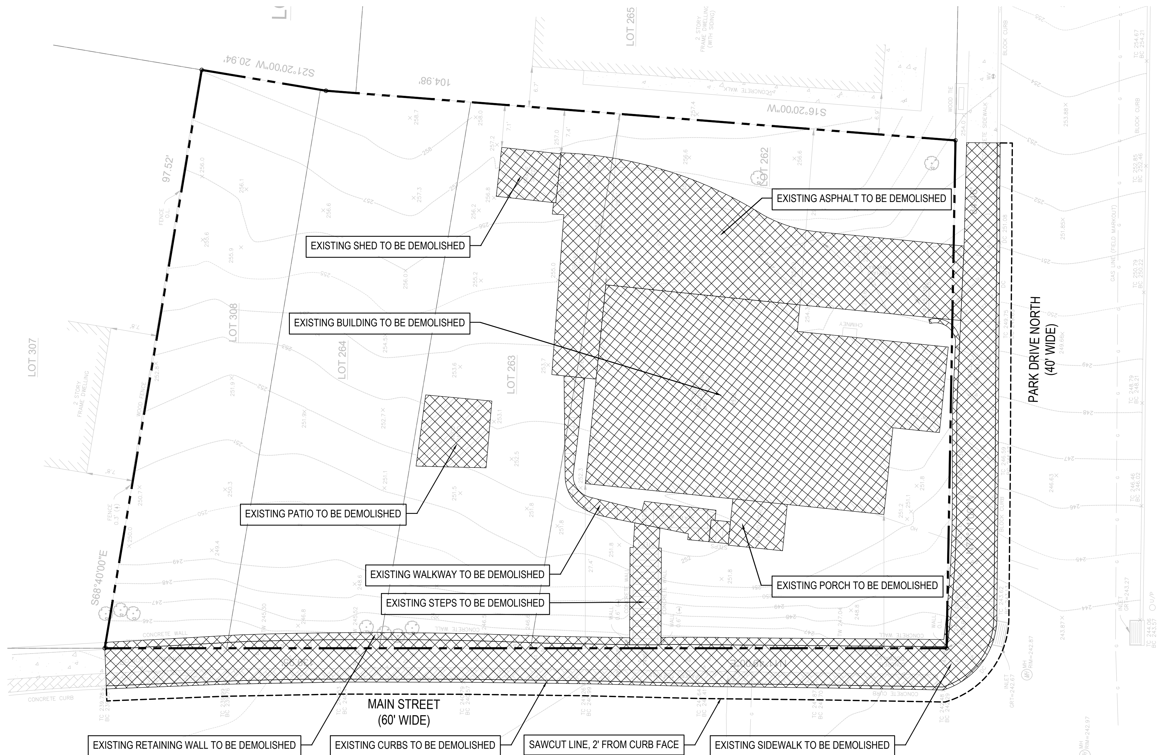
1 EXISTING CONDITIONS & DEMOLITION PLAN 1" = 10'
