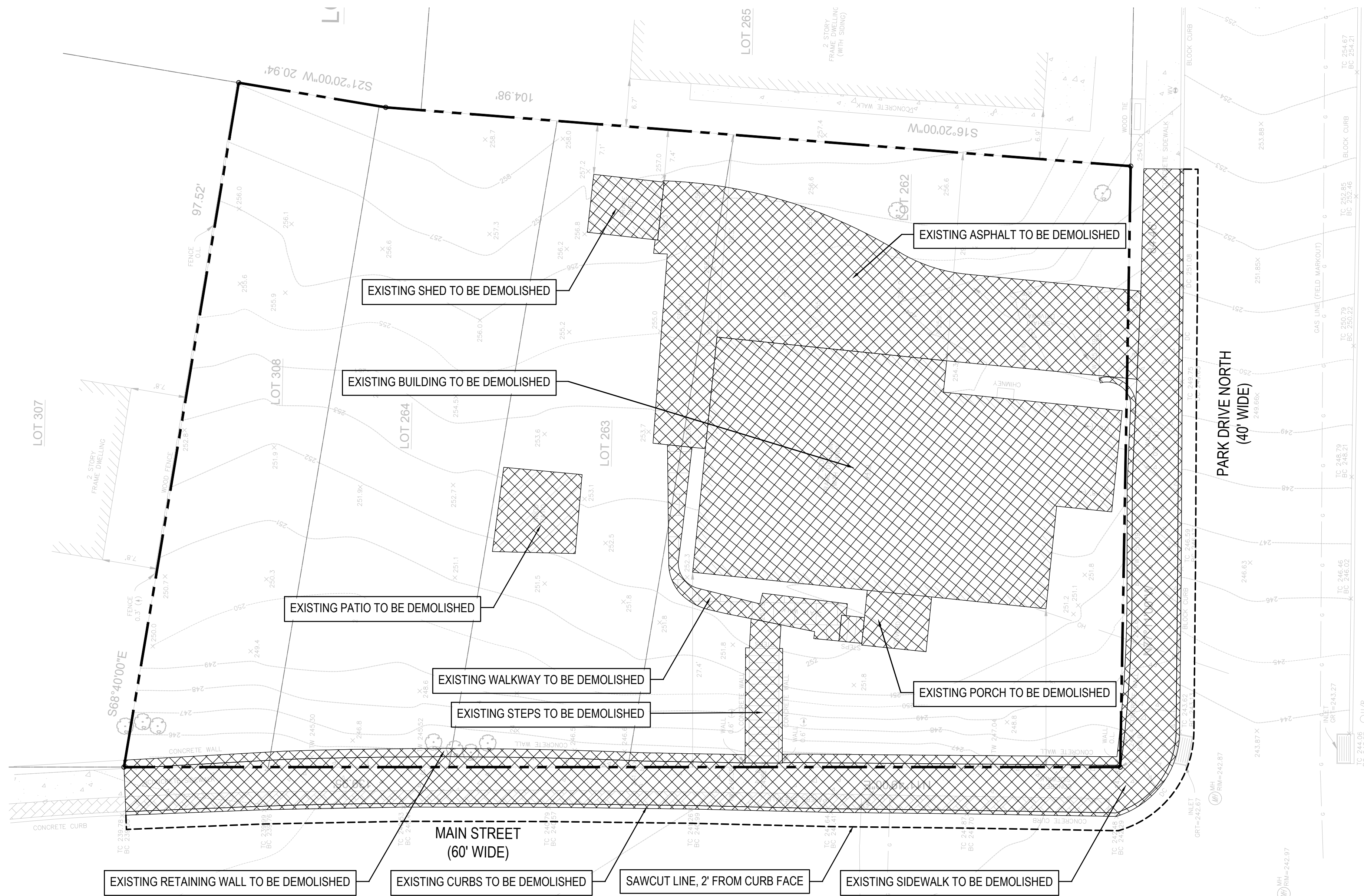
1 EXISTING CONDITIONS & DEMOLITION PLAN 1" = 10'
