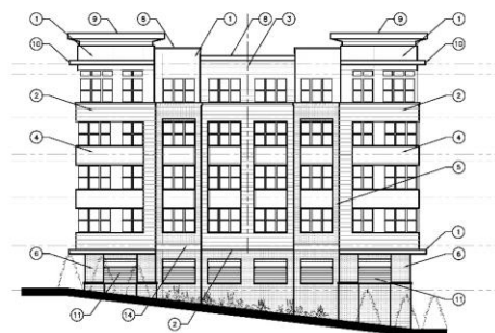
3 BUILDING B ELEVATION (NORTH) Scale: 1/16" = 1'-0"
