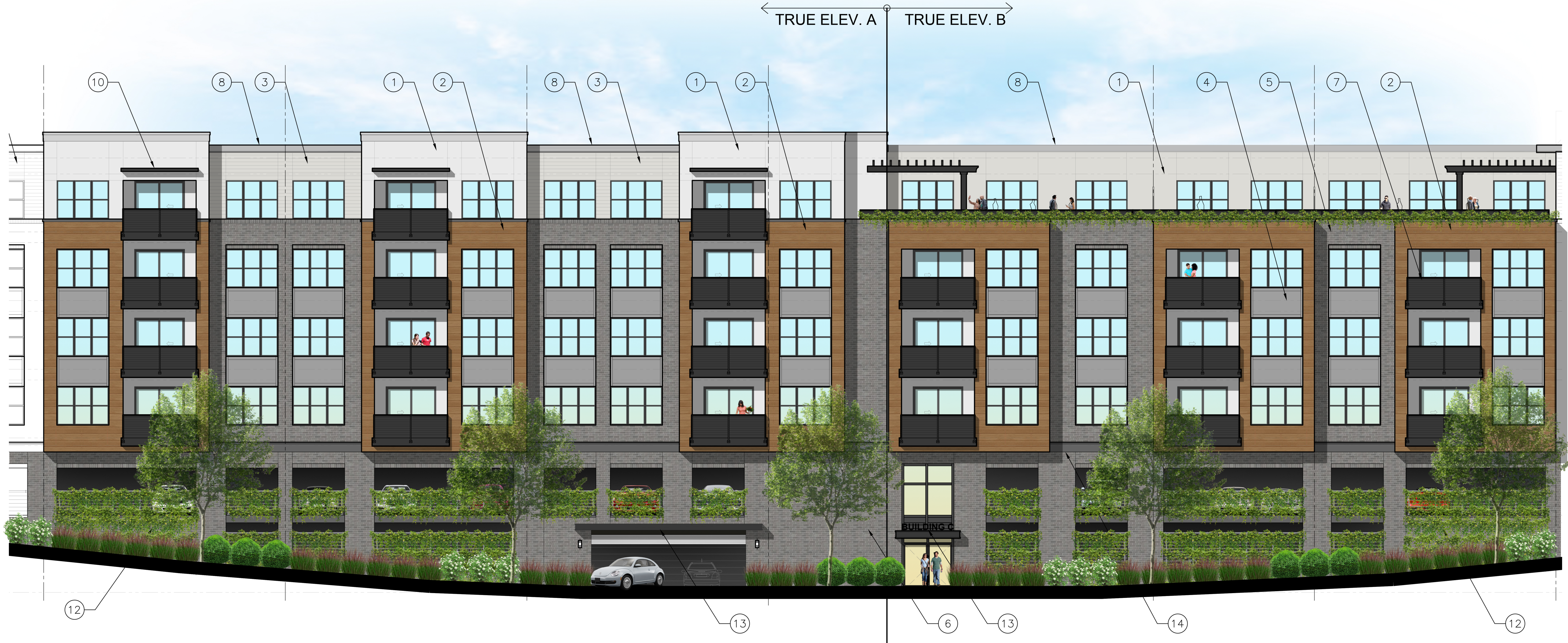
1 BUILDING C ELEVATION (SOUTH) Scale: 1/8" = 1'-0"
