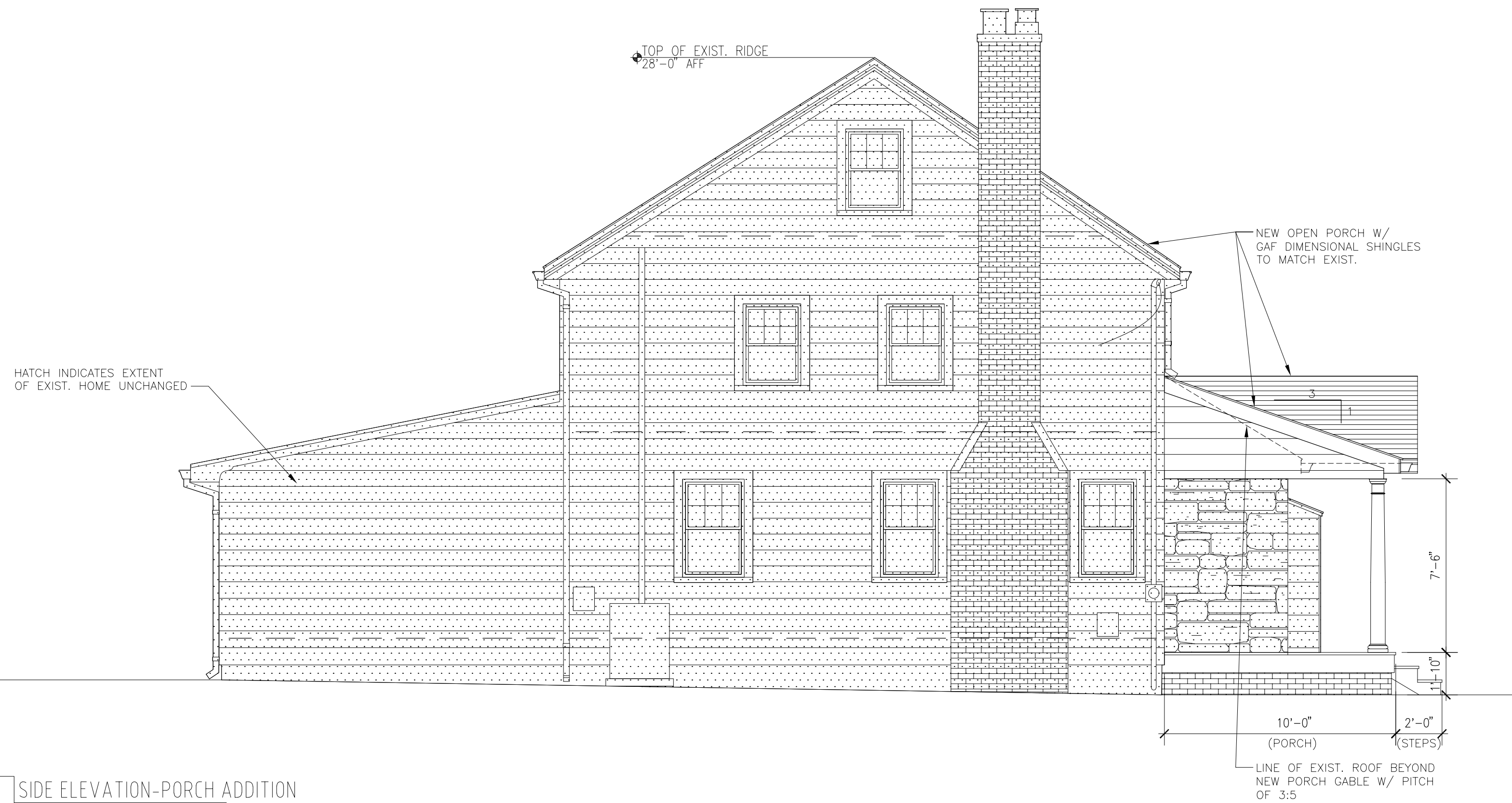
1 SIDE ELEVATION-PORCH ADDITION 1/4" = 1'-0"
