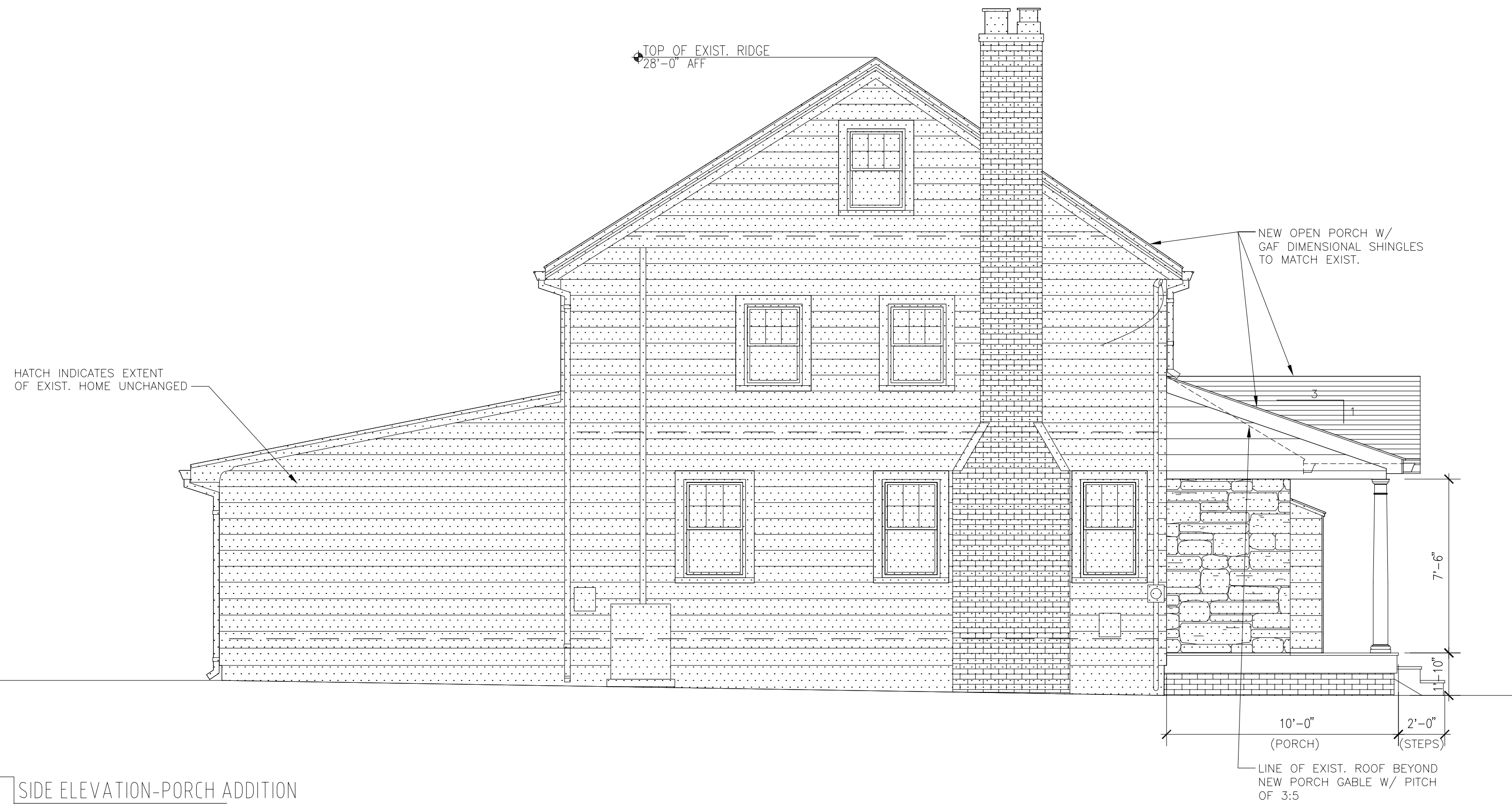
1 SIDE ELEVATION-PORCH ADDITION 1/4" = 1'-0"
