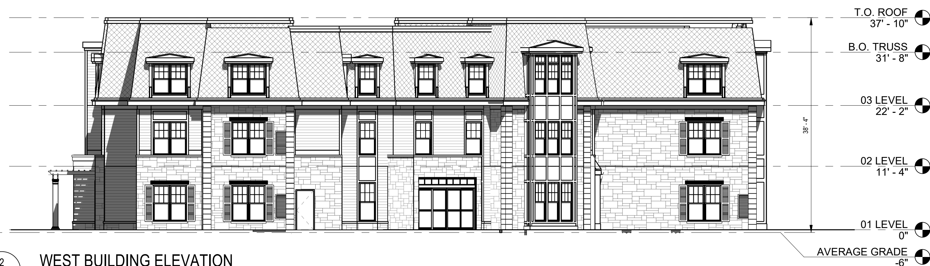
2 WEST BUILDING ELEVATION 3/32" = 1'-0"
