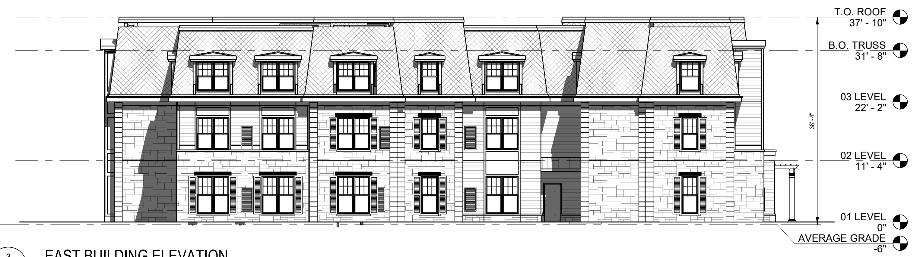
3 EAST BUILDING ELEVATION 3/32" = 1'-0"
