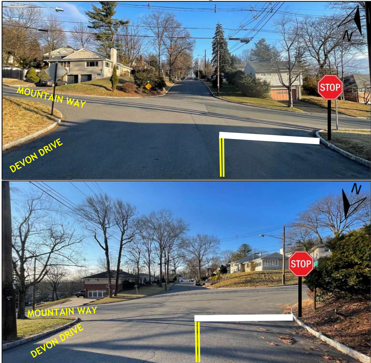
FIGURE 5 & 6 – STOP Sign Installation
